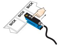
Press both the "+" and "-" buttons together, hold > 1 s and than release the teach-in buttons. The red LED flashes.
