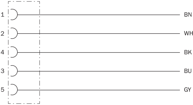
Contact assignment of the M12 female connector
