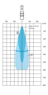
If the points named above are located in the radiation cone, reliable detection is guaranteed
