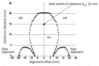
If the actuator moves laterally in relation to the surface of the sensor, a minimum distance of 4 mm must be maintained. This distance will prevent premature triggering due to the side approach areas.
