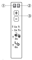
① Function signal indicator (yellow), switching output
