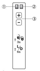
Function signal indicator (yellow), switching output
