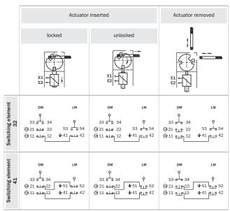
$<sup>\</sup>frac{1}{\mathbf{P}}$  Positive action N/C locking monitoring contact
