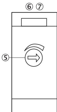
⑤ Sensing range adjustment: potentiometer, 5 turns
