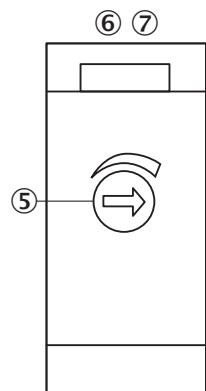
⑤ Sensing range adjustment: potentiometer, 5 turns
