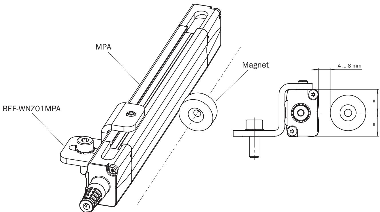
The distance from sensor to magnet must remain constant
