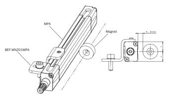
The distance from sensor to magnet must remain constant
