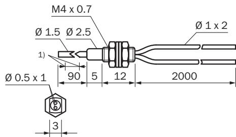
1) Flexible end tip, do not bend in this area (10 mm), bend radius R10 mm
