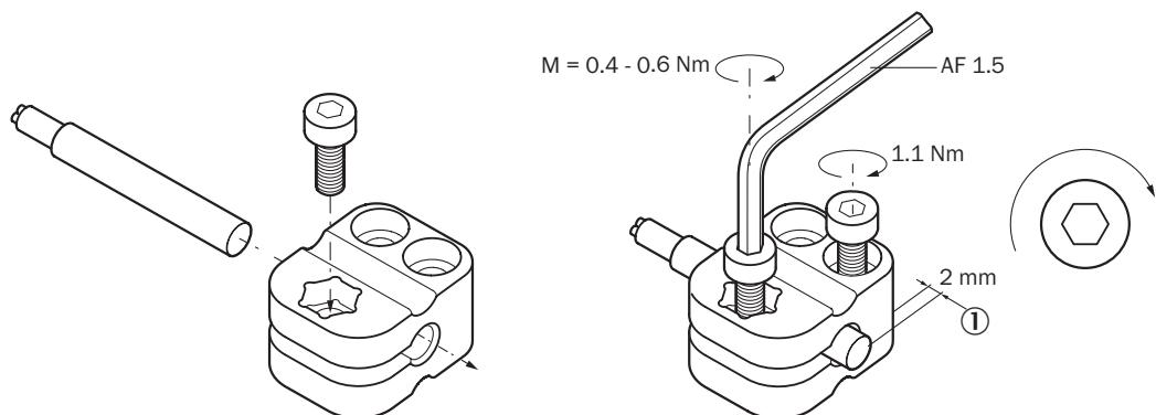
① Optimal installation position depends on the sensor model. Please check the sensor data sheet.
