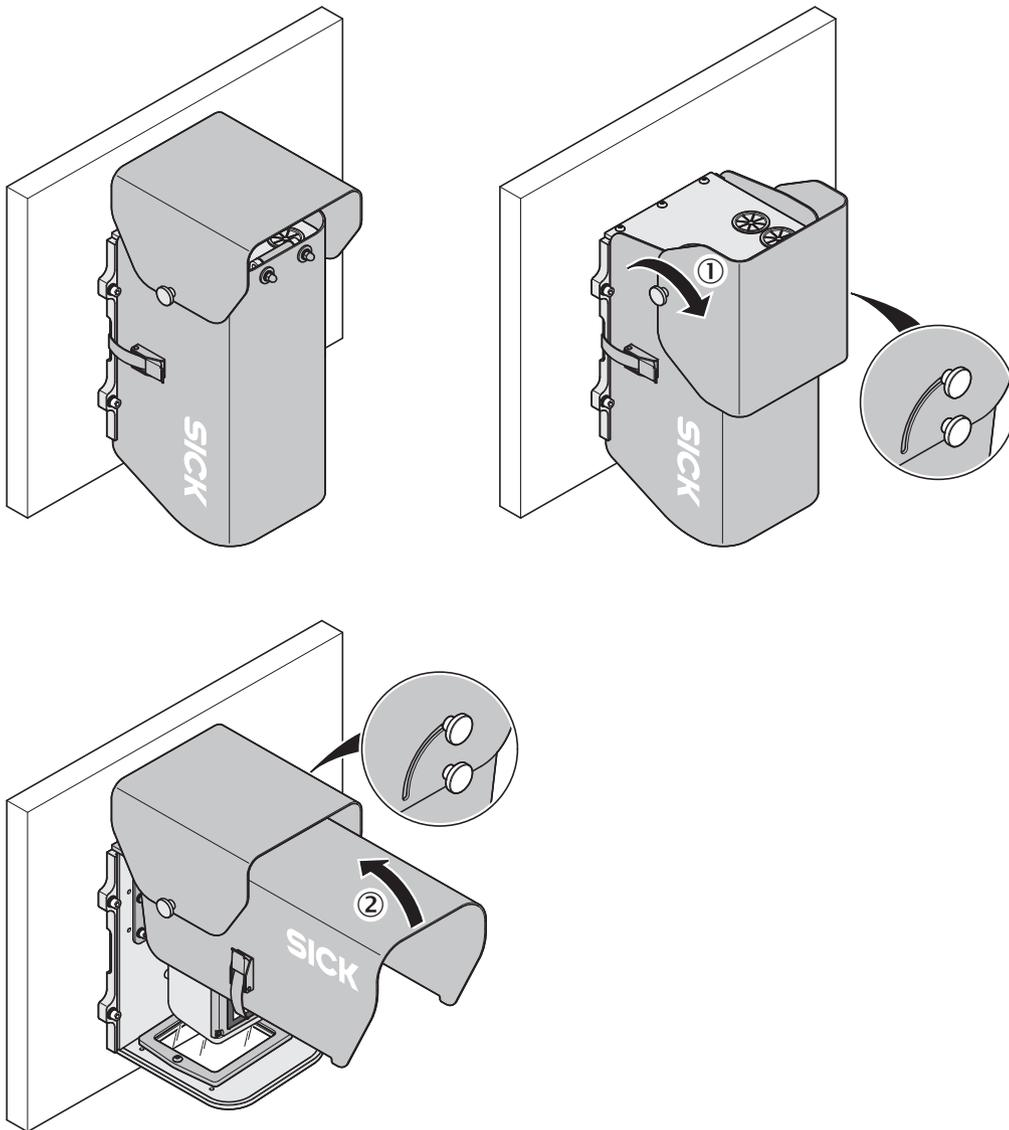
① Unscrew the knurled nut and fold the rain cover (part number 2087690) forward and over the protective housing (part number 2087695)
