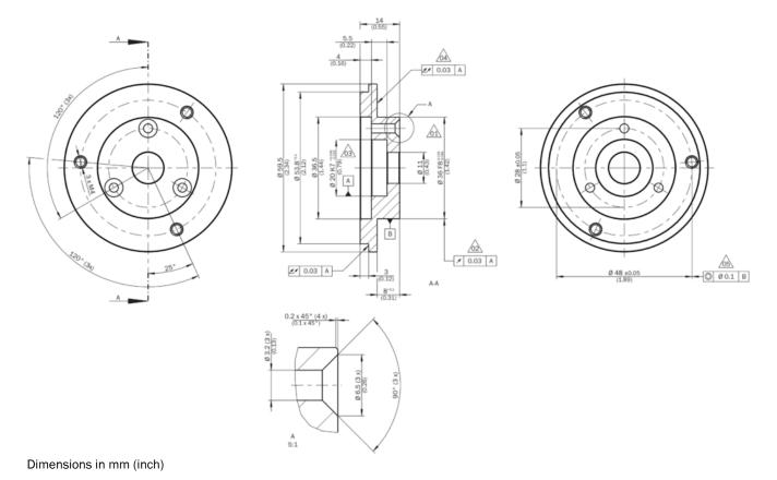
Instruction for installation Solid shaft, face mount flange with flange adapter, centering collar D20 on D36 (BEF-FA-020-036, 2072298)
