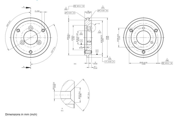
Instruction for installation Solid shaft, face mount flange with flange adapter, centering collar D20 on D50
