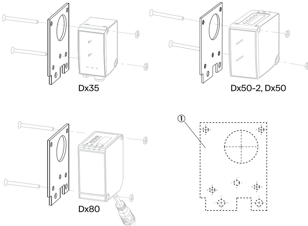
① Adapter plate (Dx35, Dx50, Dx50-2, Dx80)
