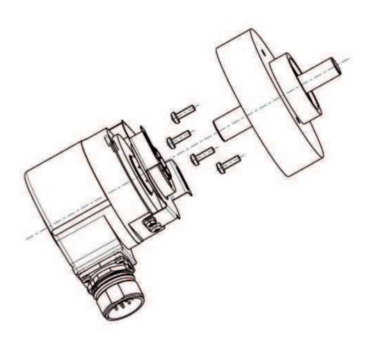
The mounting of the bearing block is performed using the threaded holes machined in the flange or with the help of a flange adapter or angled mounting bracket.
