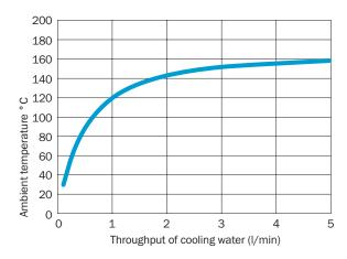
$\textcircled{\scriptsize 1}$  Temperature for cooling water 20 °C, water pressure max. 5 bar
