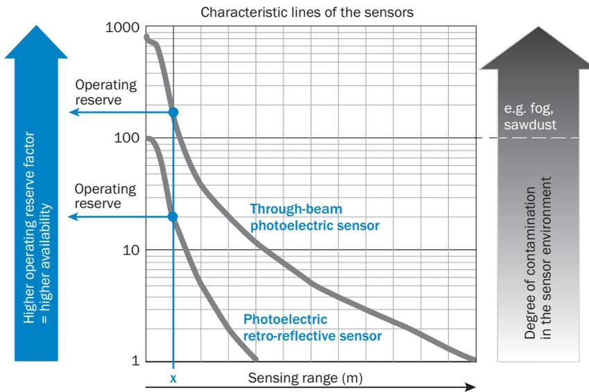
At a sensing range of „x“ the photoelectric retro-reflective and through-beam photoelectric sensors have different operating reserves (see blue arrow). The higher the operating reserve factor, the better the sensor can compensate the contamination in the air or in the light beam and on the optical surfaces (front screen, reflector), i.e. the sensor has the maximum availability, otherwise the sensor switches due to pollution although there is no object in the path of the light beam.
