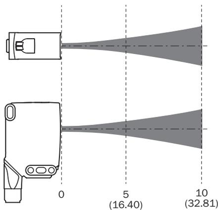
Sensing range diagram Standard reflectors
