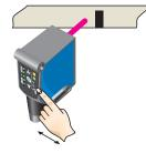
When setting the contrasts to be detected, the first LED (green) flashes in the bar graph. Press set button.
