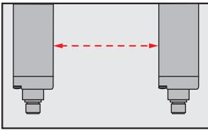
The light grid communicates via the light beams. A cable is not necessary for the optical synchronization.
