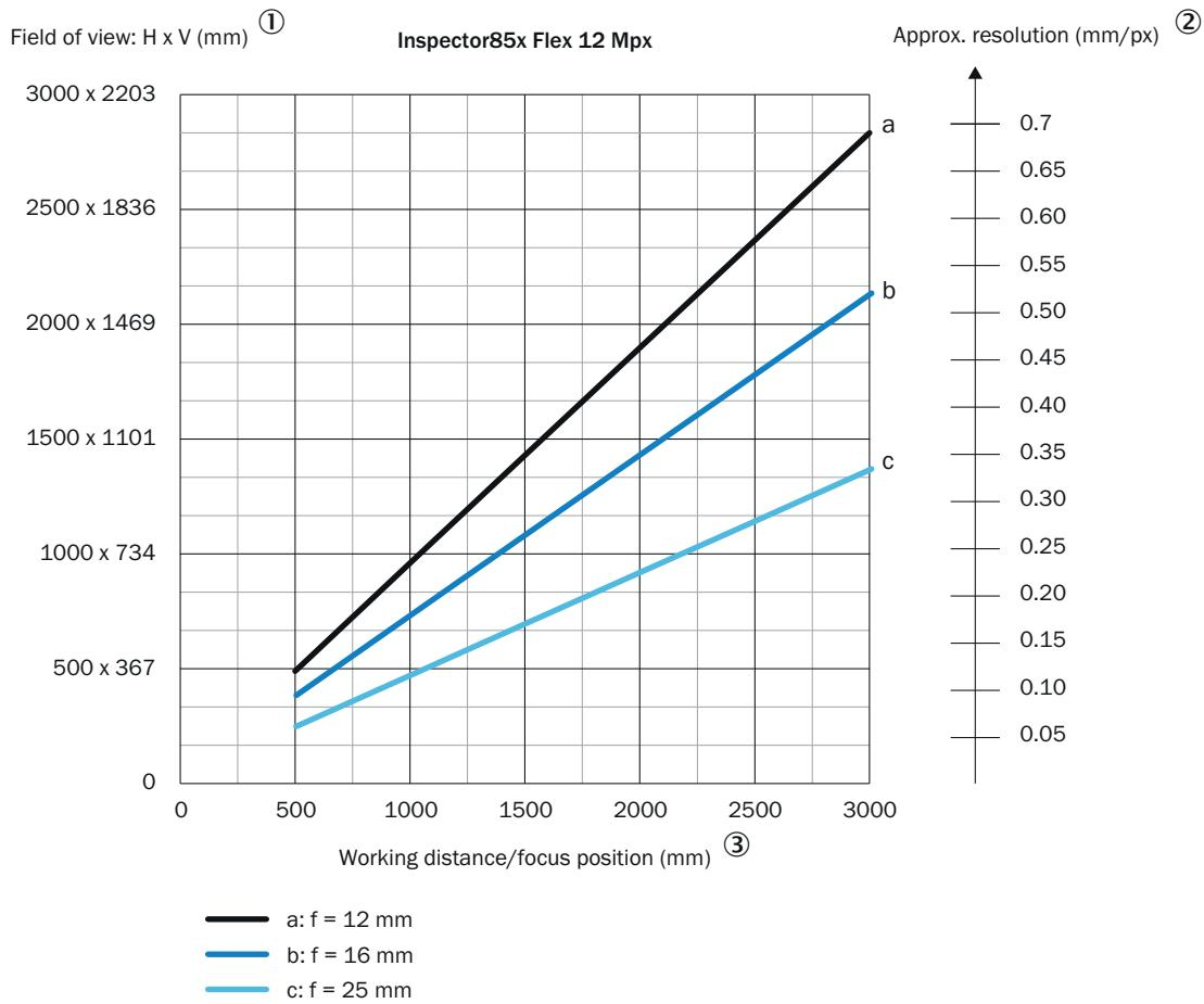
① Field of view: Horizontal x vertical in mm
