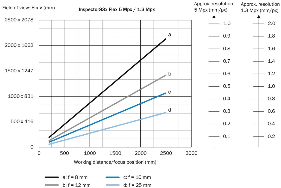
① Field of view: Horizontal x vertical in mm
