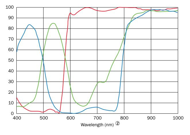
Approximate spectral transmittance for the M30 high-resolution color rows
