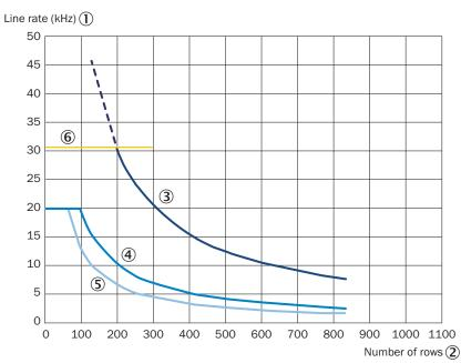
The maximum line rate is based on the number of sensor lines used
