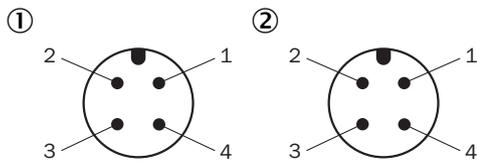
M12 male connector, 4-pin, A-coding
