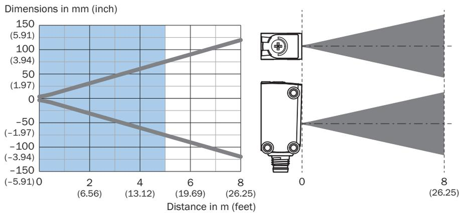
Sensing range diagram Standard reflectors
