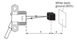
ZTB18-xxxxxx**D02**: x = 47 mm / y = 4 mm ZTB18-xxxxx**D04**: x = 93 mm / y = 8 mm ZTB18-xxxxx**D06**: x = 139 mm / y = 12 mm
