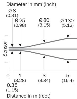
Sensing range diagram GL6 Inox, Red, Standard
