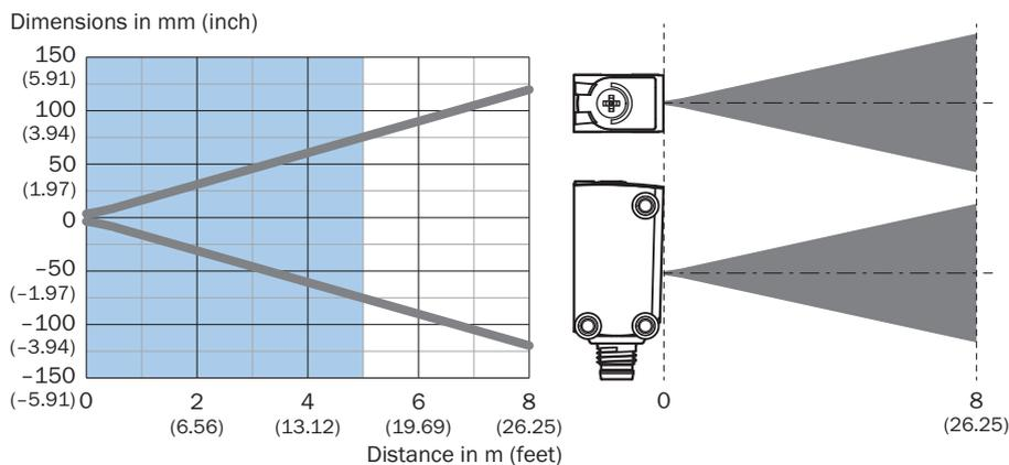
Sensing range diagram Chemical-resistant reflectors
