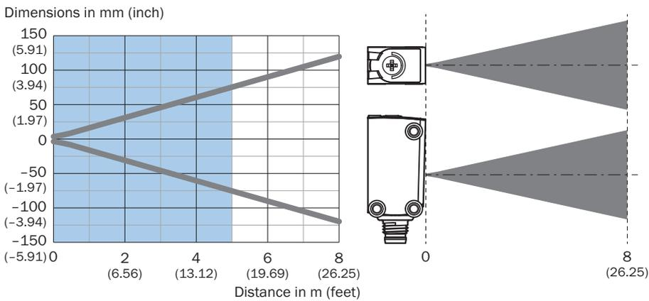
Sensing range diagram Standard reflectors
