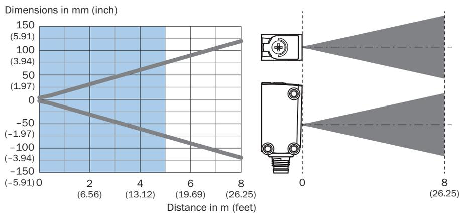
Sensing range diagram Standard reflectors
