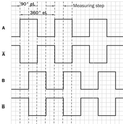
The measuring step corresponds to 90° electrical. The specified resolution, e.g. 4 μm, can only be achieved if the counter card is scanned 4 times. This ensures each signal edge within the 360° el. period (rising A, rising B, falling A, falling B) is counted.
