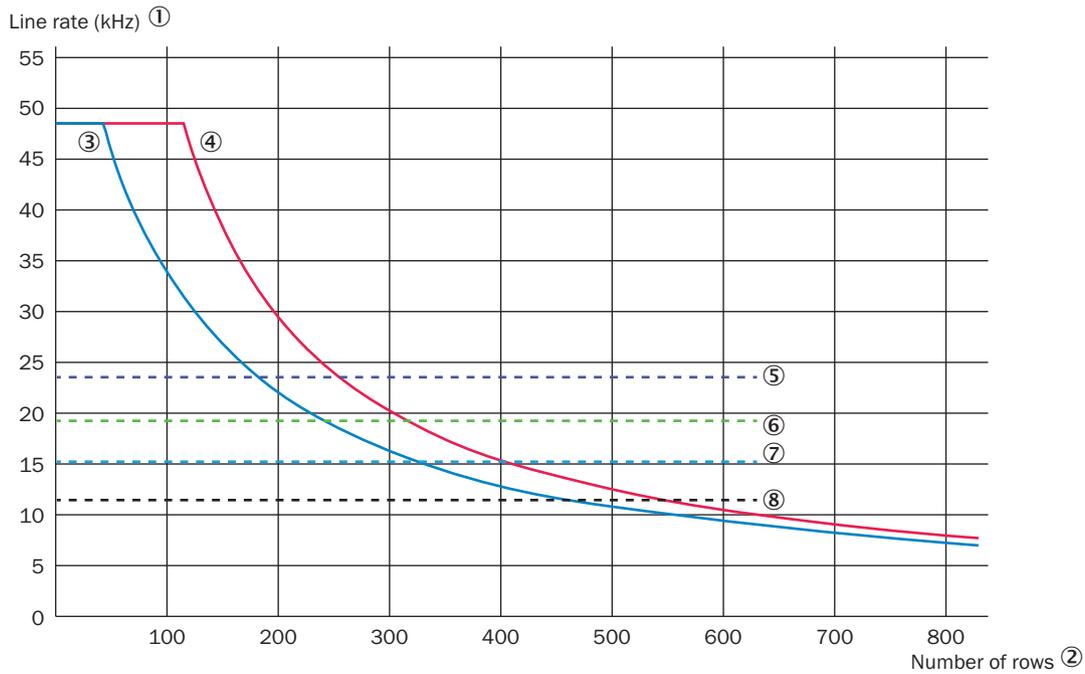
The maximum line rate is based on the number of sensor lines used
