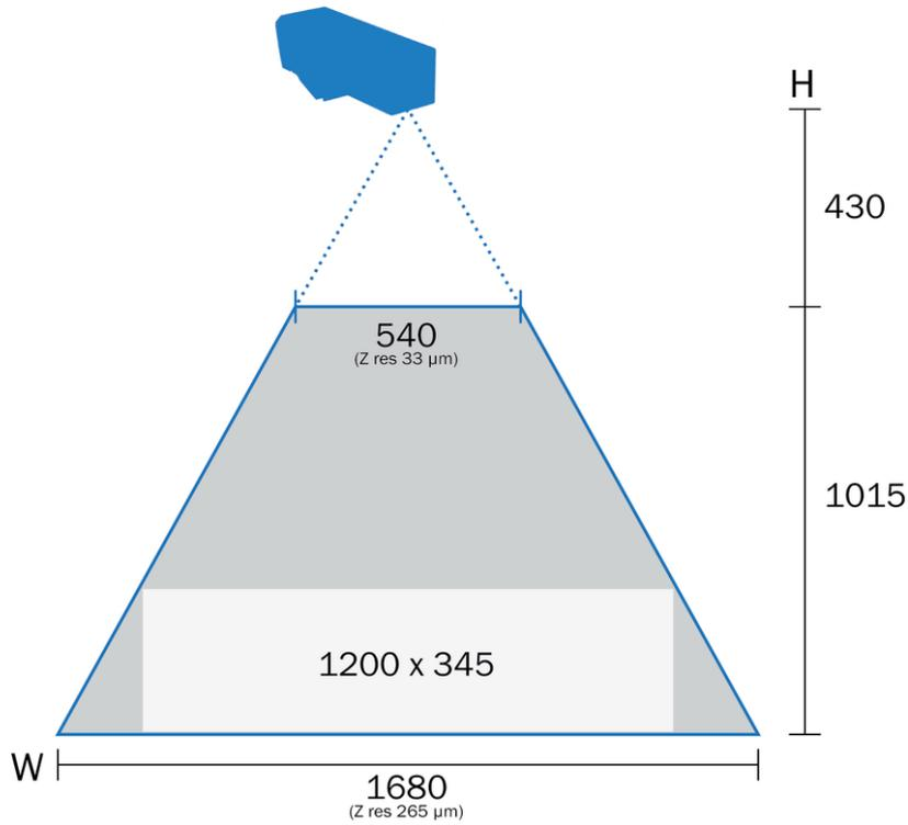
Characteristic curve Width of the field of view via the Z position
