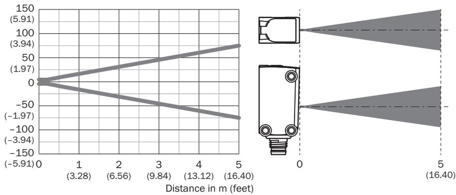
Sensing range diagram Standard reflectors
