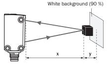
Black object (6 % remission factor) Set sensing range  $x=150\ mm$  Needed minimum distance to white background  $y=5.5\ mm$
