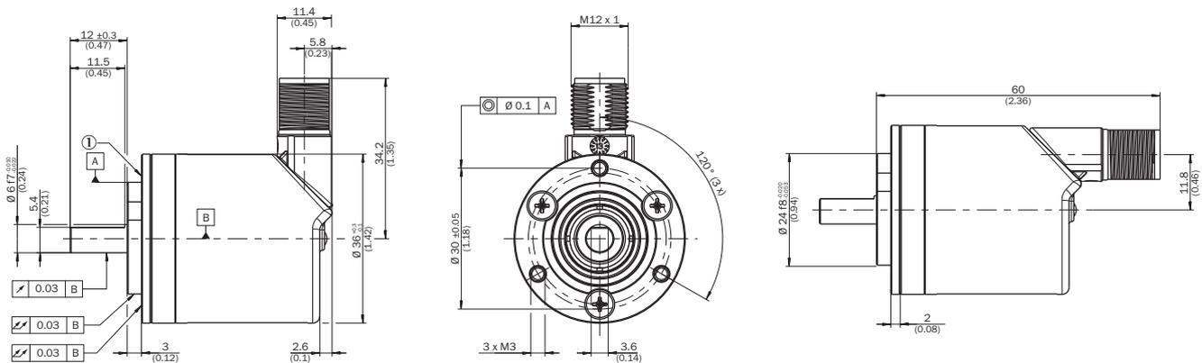
order example for 6 mm shaft diameter: AHx36x-S3xx0xxxxx + BEF-FA-020-024 (adapter is not pre-assembled)
