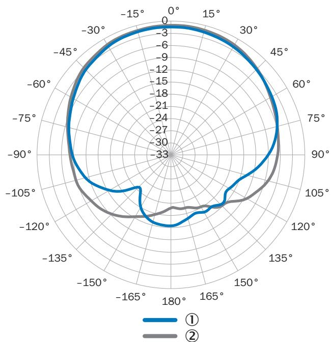
measured antenna gain in dBi at 866.5 MHz, LHCP (left-hand circularly polarized)
