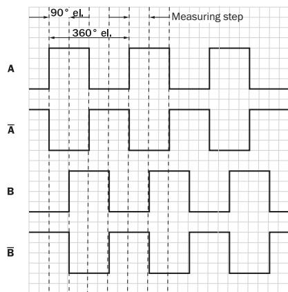
The measuring step corresponds to 90° electrical. The specified resolution, e.g. 4 µm, can only be achieved if the counter card is scanned 4 times. This ensures each signal edge within the 360° el. period (rising A, rising B, falling A, falling B) is counted.
