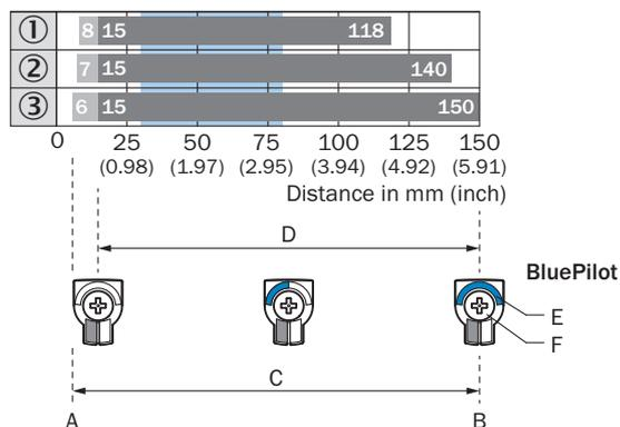
A = Sensing range min. in mm
