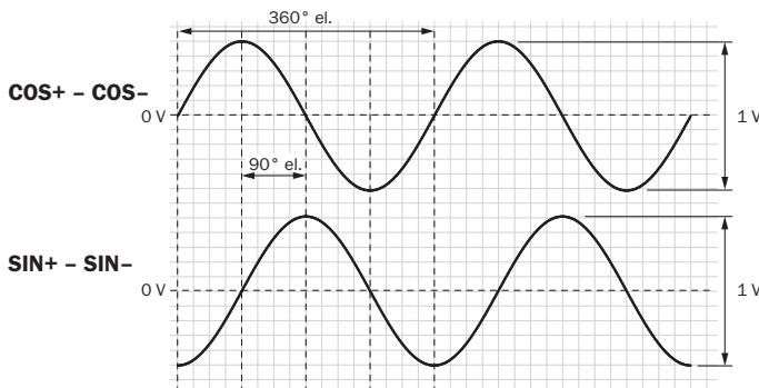
For clockwise shaft rotation, looking in direction "A" (see dimensional drawing)
