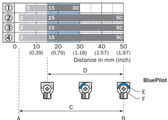
A = Sensing range min. in mm
