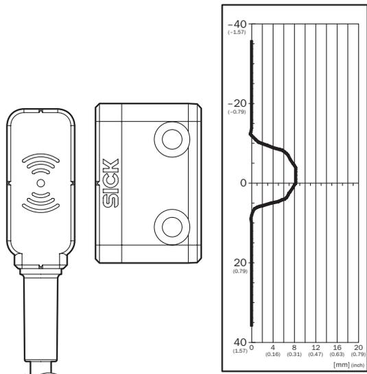
assured switch on distance  $S_{ao}$  6 mm
