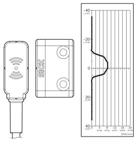
assured switch on distance  $S_{ao}\,6\,mm$
