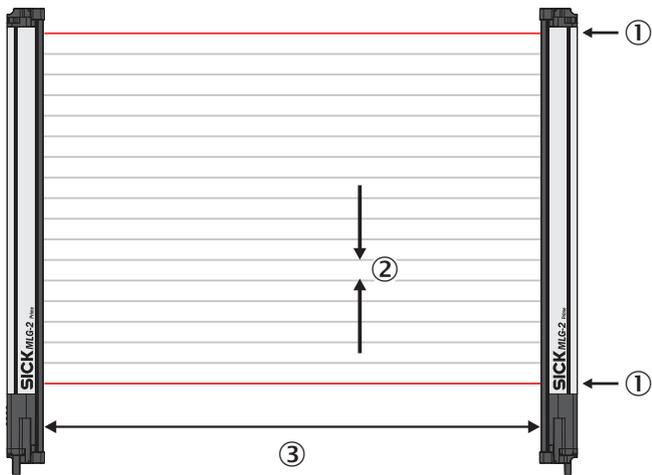
The sender and receiver synchronize with each other optically, so no electrical connection is necessary. For this reason, either the first or the last beam of the automation light grid must remain clear. If both beams are interrupted, no measurements can be taken.
