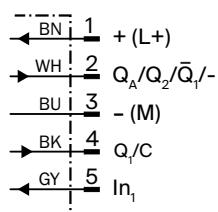
Supply voltage & I/O: plug, 5-pin
