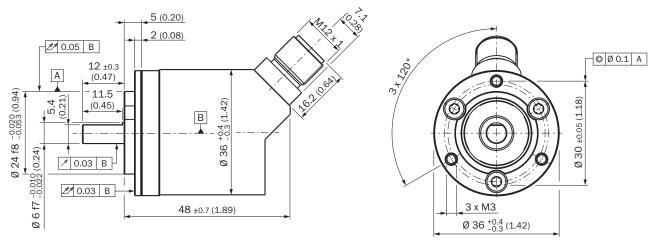
order example for 6 mm shaft diameter: AHx36I-S3xx0xxxxx + BEF-FA-020-024-I (adapter is not pre-assembled)
