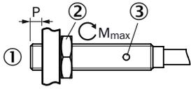
Mounting using two mounting nuts
