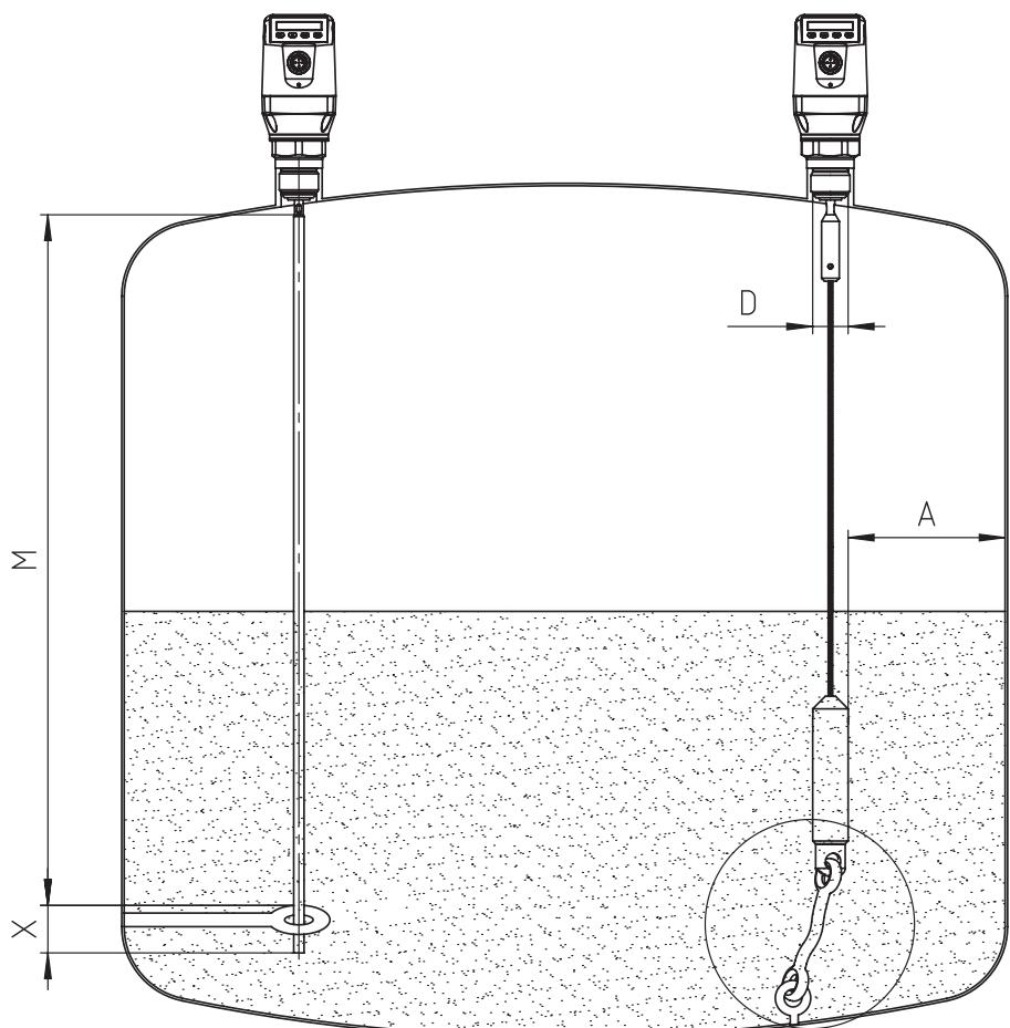
**Mono rod probe mounted in metal tank**
