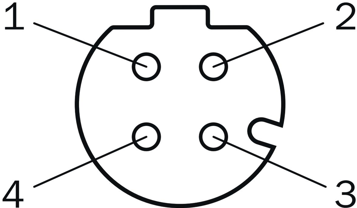
M12 female connector, 4-pin, D-coded
