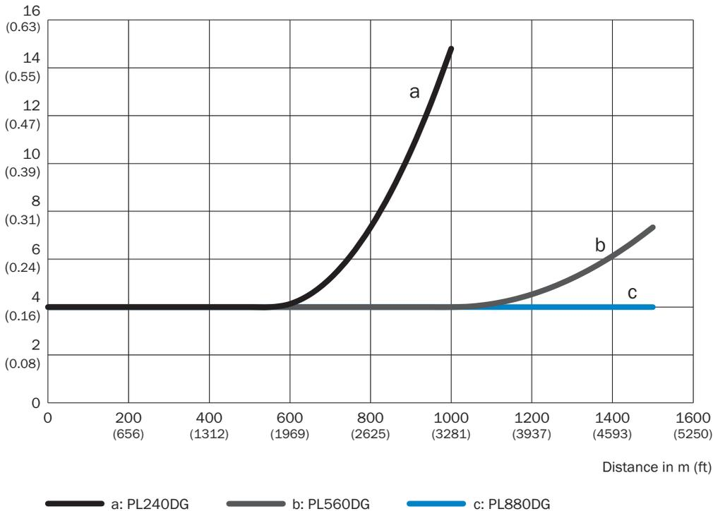
Measurement accuracy Typically DL1000, x-axis: Distance, y-axis: Typical measurement accuracy
