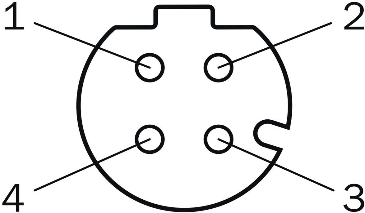
M12 female connector, 4-pin, D-coded
