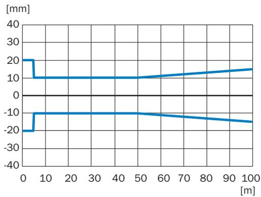
Measurement accuracy Typically DL1000, x-axis: Distance, y-axis: Typical measurement accuracy
