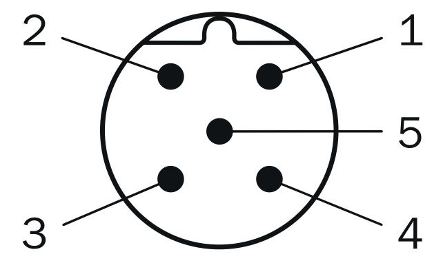
Connector M12, 5-pin, A-coded
