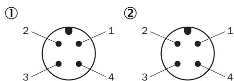
M12 male connector, 4-pin, A-coding
